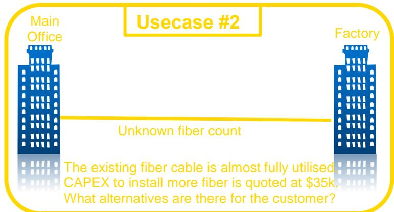
**Solution:** The customer can use one of their spare fibers to deploy a passive CWDM solution between the main office and the plant facility. In this instance an 8# passive CWDM solution would be ideal as that would allow for 8 spare channels for future growth as well as the use of the remaining spare fibers.
